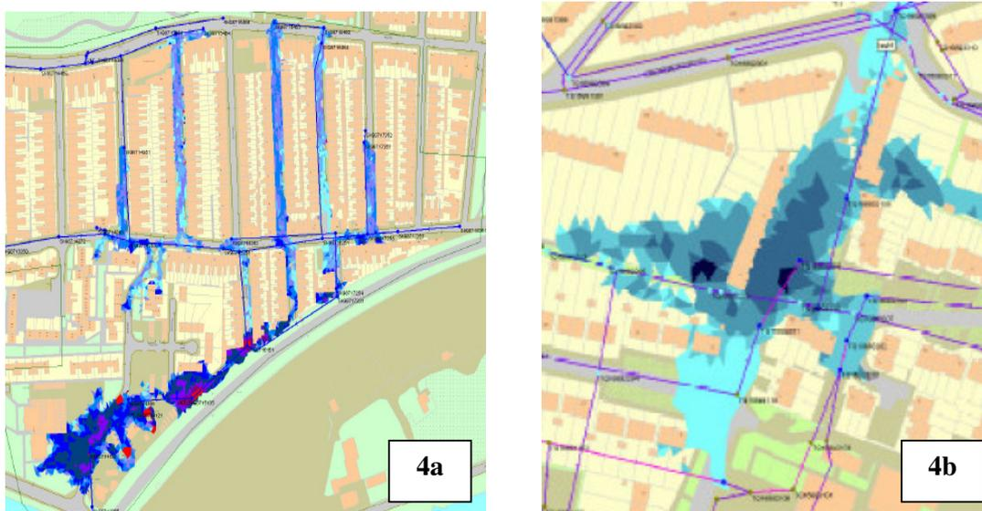
**Figure 4. Modelled Surface Flow Paths During an Extreme Event.**
