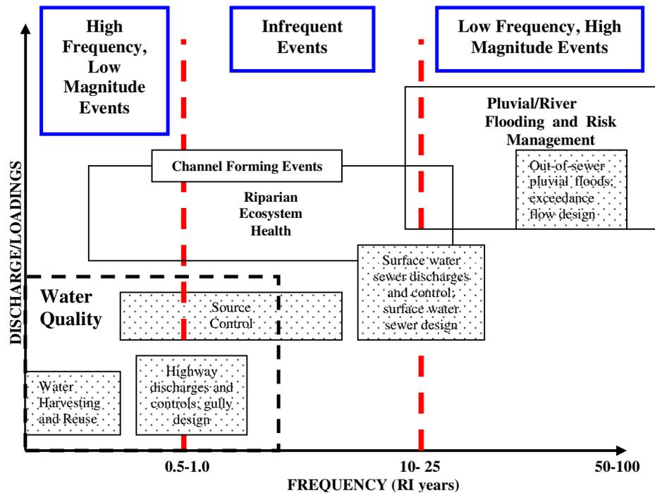
**Figure 1. Stormwater Management Planning Scales and Issues.**
